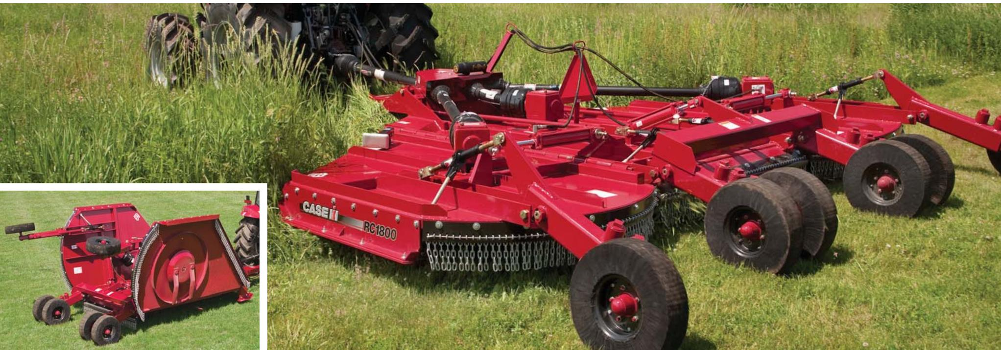
**A smooth underdeck design** allows cut material to move unrestricted, reducing rust hazards on Case IH rotary cutters.
