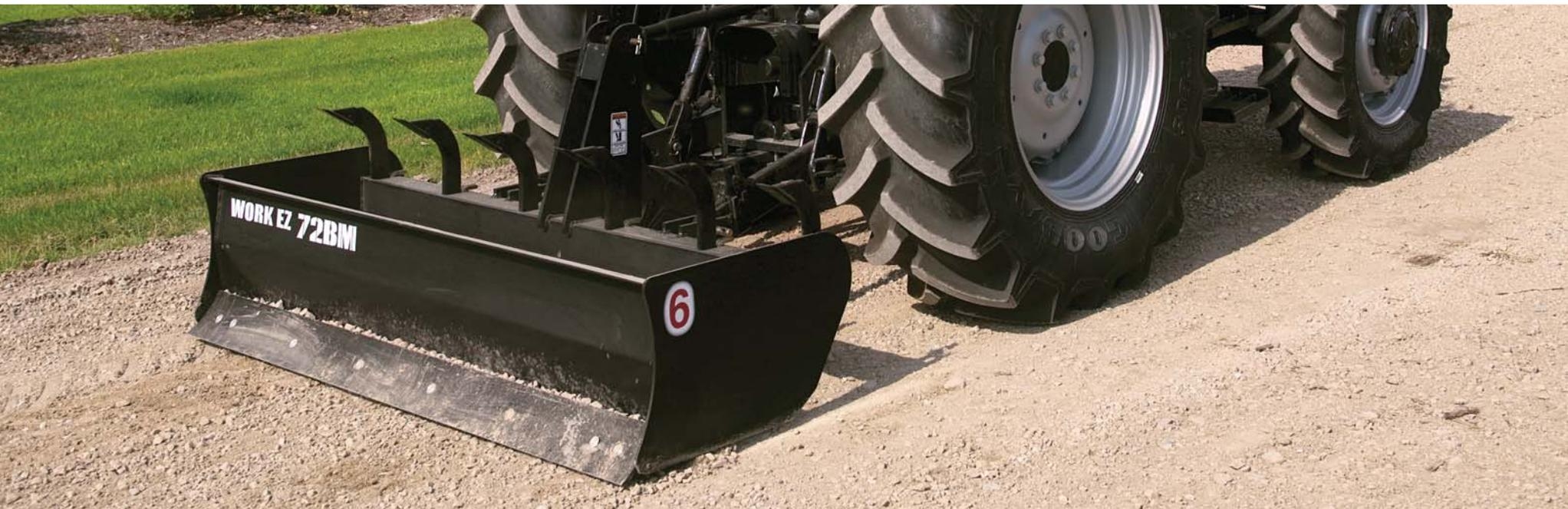
**Work EZ box blades** from Case IH include heat-treated, easily adjustable scarifier shanks with replaceable tips to rip through hard-packed soils.
