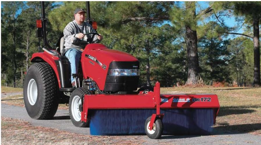
**Case IH BR Series Quick-Attach front rotary brooms** can be manually angled from 0 - 25 degrees. Or change the broom angle from your tractor seat with optional hydraulic angling.
