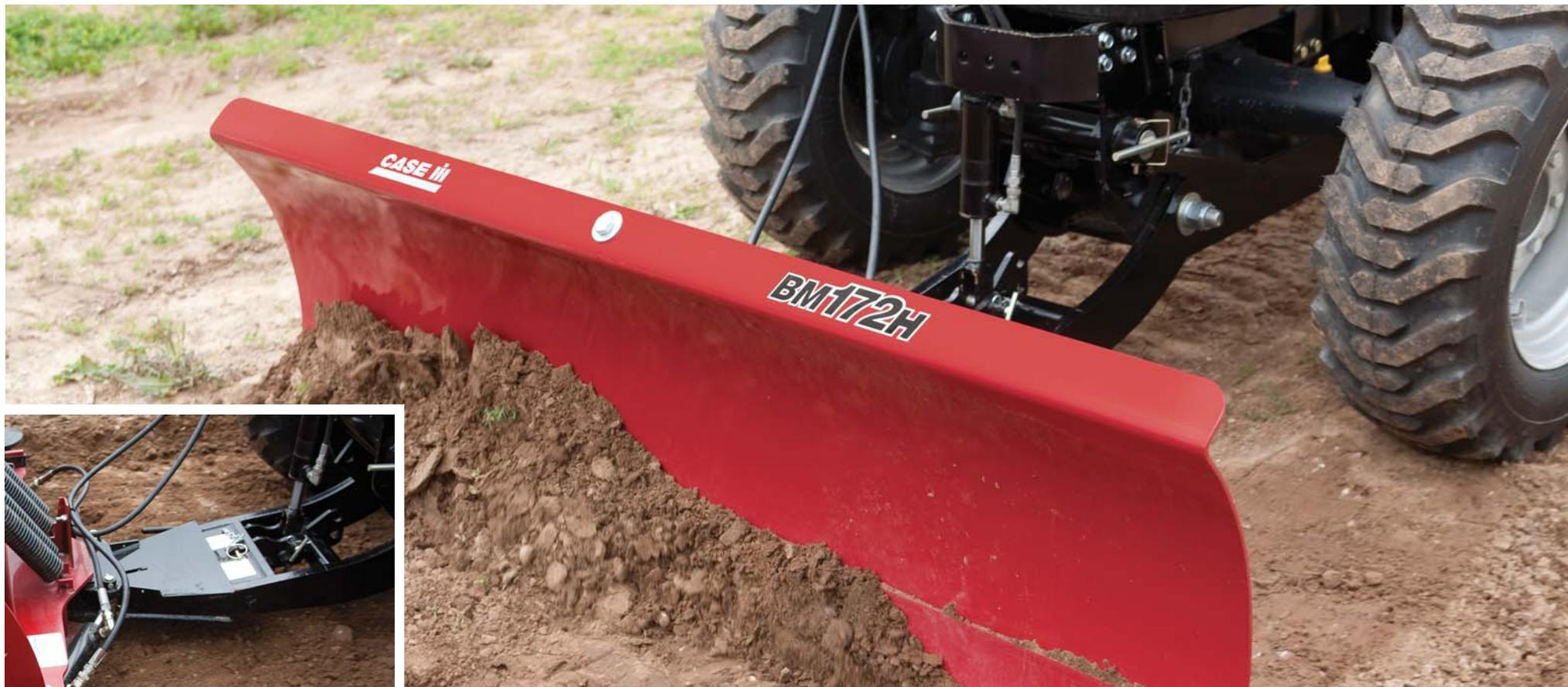
Case IH **Quick-Attach front blades** bolt on for long life and easy maintenance, and are easily attached and removed without tools.
