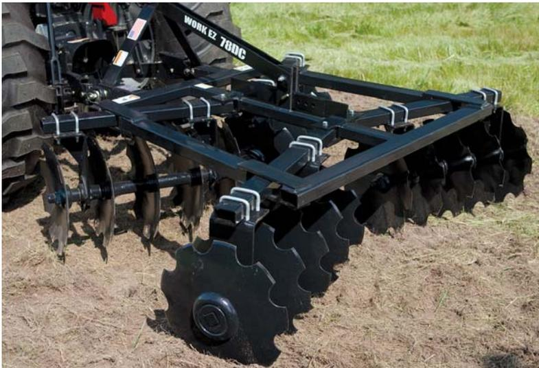
The Work EZ disk harrow from Case IH offers a cutting width of 70 in. for tractors up to 70 hp.
