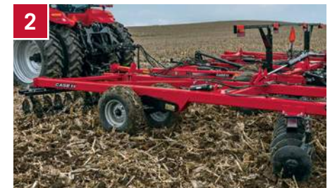
2 Disk gang depth: slice, cut and bury residue to the producer's desire.
