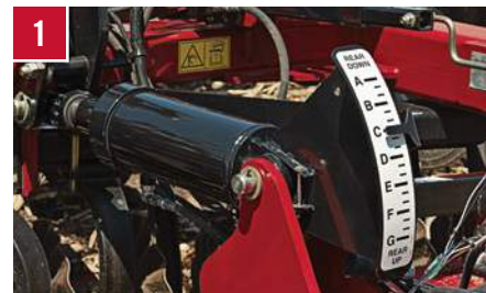
1 Hydraulic fore/aft control: maintain consistent agronomic output.
