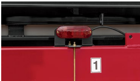
Tank full indicator lights.
