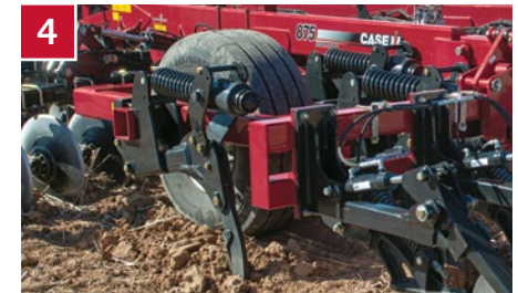
4 Shank depth: target the compaction layer
