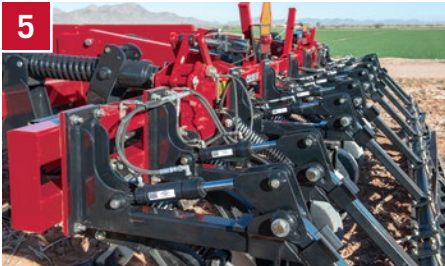
5 Crumbler pressure: achieve consistent clod sizing
